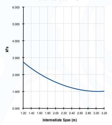
Note: The intermediate spans shown in the graphs above are based on G300 Steel as the base metal. To calculate end spans please multiply the intermediate span calculated by 0.66. Spans are based on restricted access. For alternative metals please contact your local Metalcraft branch.
