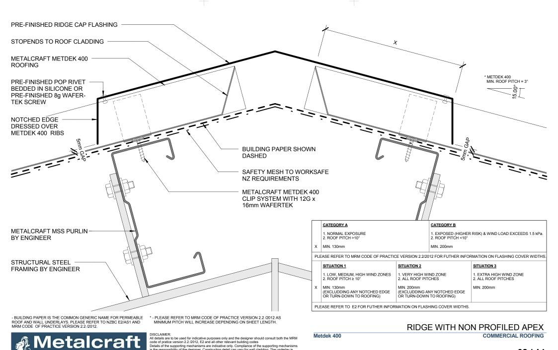
is the responsibility of the designer. Construction detail can vary for wall cladding. The underlay is
