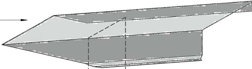
(3) PRE-FINISHED 3D SADDLE FLASHING
