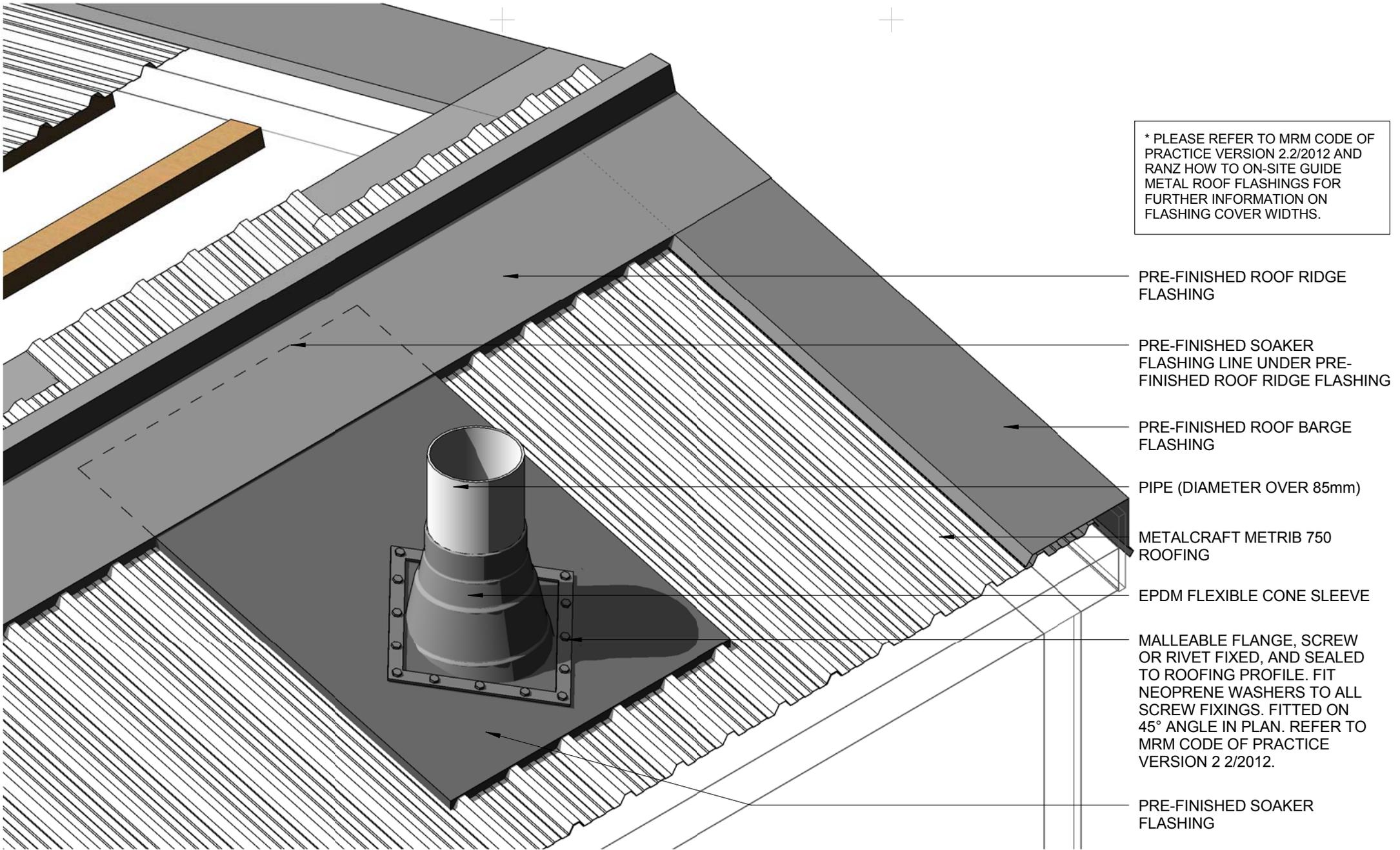
\* PLEASE REFER TO MRM CODE OF PRACTICE VERSION 2.2/2012 AND RANZ HOW TO ON-SITE GUIDE METAL ROOF FLASHINGS FOR FURTHER INFORMATION ON FLASHING COVER WIDTHS.
