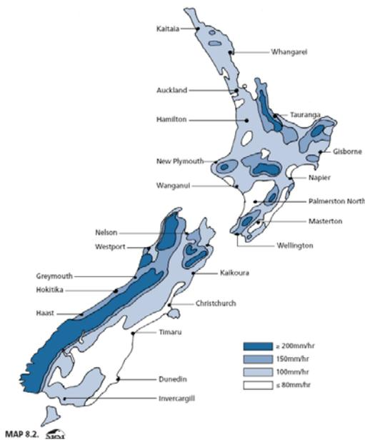
The information above has been referenced from the NZ Metal Roof and Wall Cladding Code of Practice Version 2 section 8. This document does not constitute design recommendations and is intended to highlight issues around roof drainage design. For further information or clarification of the information above please contact Metalcraft.
