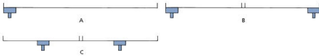
Based on a roof with the same catchment area for each example, Type B would require one half the gutter capacity of Type A whilst Type C would require one quarter the capacity. The downpipe capacity required for both Types B and C would be half that of A.
