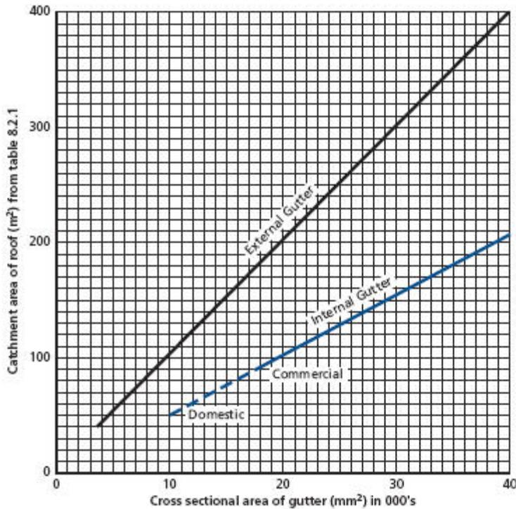
These graphs are suitable for roof pitches up to 10° and a rainfall intensity of 100mm/hr. For other roof pitches and rainfall intensities see the example.
