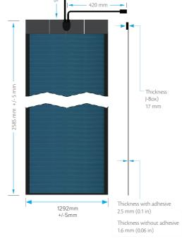
Thickness with adhesive 2.5 mm (0.1 in) Thickness without adhesiv 1.6 mm (0.06 in)
